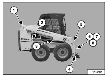
The grease fitting locations **[Figure 271]** are shown in more detail in the following figures.
