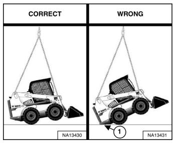
Attach cables or chains to lift eyes [Figure 160].
