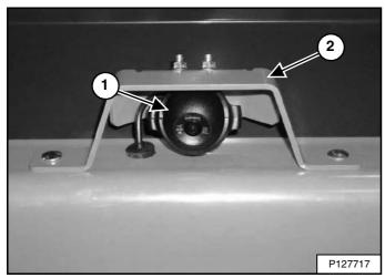
The rear camera (Item 1) is located inside a bracket (Item 2) **[Figure 21]** mounted on top of the rear door.
