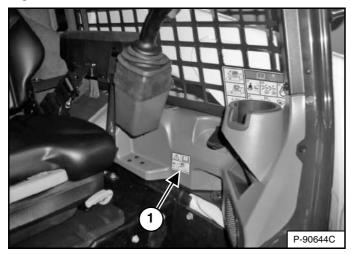
Inspect for damaged or missing back-up alarm decal (Item 1) [Figure 174]. Replace if required.
