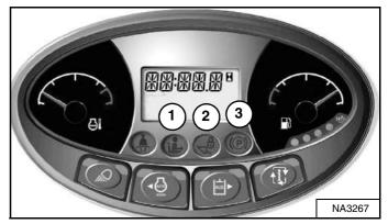
There are three display lights (Items 1, 2, and 3) **[Figure 33]** located on the left instrument panel that must be OFF to fully operate the machine.
