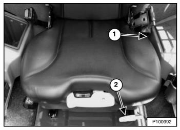
Pull the lever (Item 1) **[Figure 120]** up to adjust the angle of the seat back.
