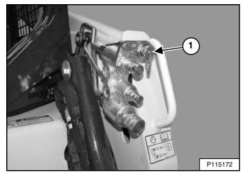
Connect the attachment electrical harness to the attachment control device (Item 1) [Figure 113].
