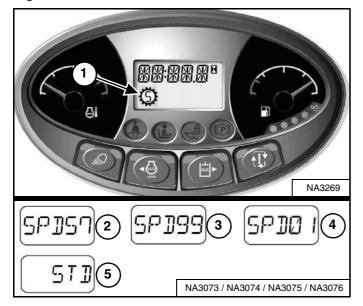
The Speed Management icon (Item 1) [Figure 83] will appear in the display and remain on until the Speed Management button is pressed again or the machine is turned off.
