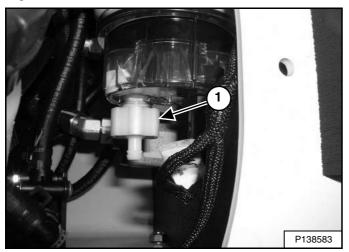
Attach a 9 mm (3/8 in) hose to the drain (Item 1) **[Figure 206]** at the bottom of the main fuel filter. Route the other end of the hose to a container.
