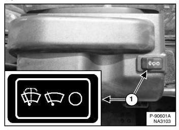
Press the left side of the switch (Item 1) **[Figure 29]** to start the front wiper (press and hold for washer fluid). Press the right side of the switch to stop the wiper.
