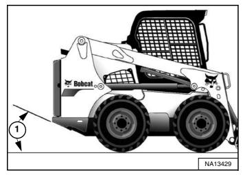
NOTE: The loader should be lifted as close to horizontal as possible, but at no time should the angle of the suspended loader exceed the departure angle (Item 1) [Figure 159] provided in the specifications section. (See Machine Dimensions on Page 211.)
