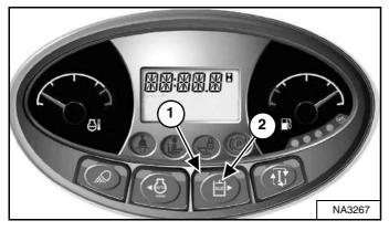
Press the Auxiliary Hydraulics button (Item 2) **[Figure 100]** once to activate the auxiliary hydraulics.
