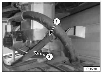
Remove the clamp (Item 1). Pinch off the hose (Item 2) **[Figure 247]** near the fitting and disconnect hose from the fitting.
