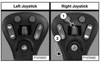
After activating the auxiliary hydraulics, press the Continuous Flow Control switch (Item 2) [Figure 103] or [Figure 104] to allow constant auxiliary hydraulic fluid flow to the front female coupler (female coupler is pressurised). (EXAMPLE: Operate a backhoe.)
