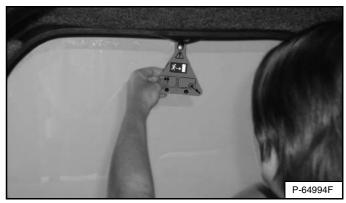
Pull on the tag on the top of the rear window to remove the rubber cord **[Figure 61]**.
