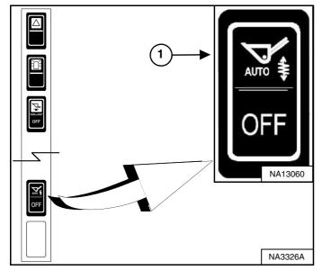
Press the top of the Automatic Ride Control switch (Item 1) **[Figure 97]** on the left switch panel to engage the automatic ride control function.
