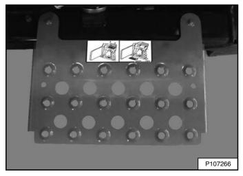
A maintenance platform **[Figure 219]** is available from your Bobcat dealer to facilitate access when cleaning the engine cooling system.
