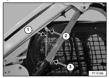
Remove the retaining pin (Item 3) [Figure 171] from the lift arm support device.
