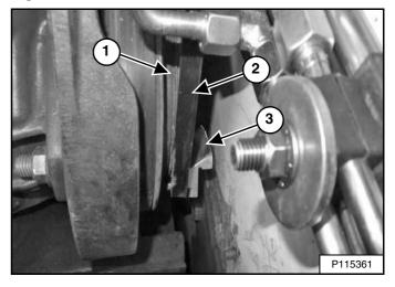
Install the belt on the air conditioning compressor pulley and start the belt (Item 2) and the belt tool (Item 3) on the front side of the hydraulic pump pulley (Item 1) [Figure 266].
