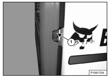
Reach into the slot on the right side of the rear door and pull the latch handle (Item 1) **[Figure 185]**. Pull the rear door open.
