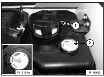
Check the fluid level in the sight gauge (Item 2). Keep the fluid level within the operating range (Inset) [Figure 242].
