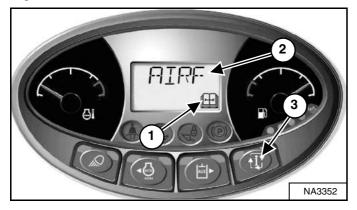
Replace the air filters only when necessary. The service indicator (Item 1) will FLASH. Press the Information button (Item 3) until the display screen shows the service codes. Service code **[AIRF]** (Replace Engine Air Filter) or **[M0117]** (Air Filter Plugged) will show in the display screen (Item 2) **[Figure 199]** when air filter replacement is necessary.
