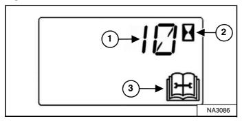
During machine operation, a 2 beep alarm will sound when there are less than 10 hours until the next planned maintenance.
