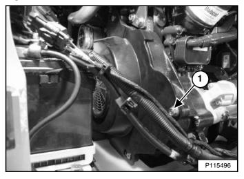
Install the drive belt shield bolt (Item 1) [Figure 270].
