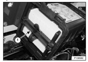
Remove the outer filter (Item 1) [Figure 201] and discard.
