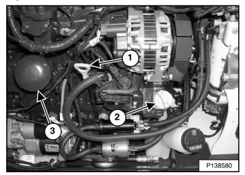
Remove the oil filter (Item 3) [Figure 218] and clean the filter base.
