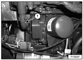
Install the coolant hose (Item 1) [Figure 230] onto the engine oil cooler fitting and install the clamp.
