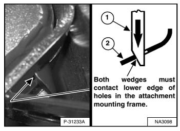
The wedges (Item 1) **[Figure 285]** must extend through the holes in the attachment mounting frame.
