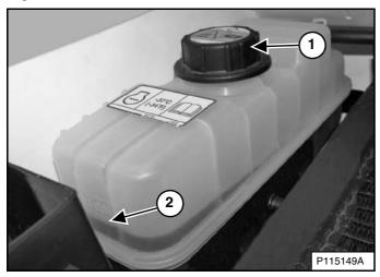
Coolant must be between the top and bottom level markers (Item 2) **[Figure 226]** when the engine is cold.
