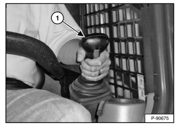
The joystick that controls drive and steering is on the left side in front of the seat (Item 1) **[Figure 75]**.
