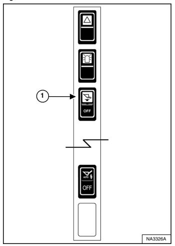
Press the top of the Bucket Positioning switch (Item 1) **[Figure 96]** on the left switch panel to engage the bucket positioning function. The amber light in the switch will turn ON.
