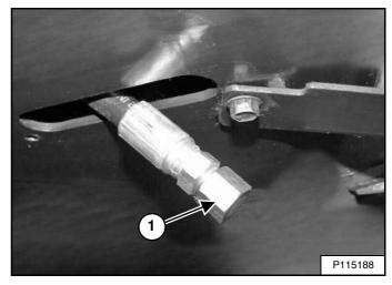
Remove the oil drain cap (Item 1) [Figure 217] from the oil drain hose and drain the oil into a container. Recycle or dispose of used oil in an environmentally safe manner.
