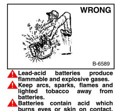
burns eyes or skin on contact. Wear protective clothing. If acid contacts body, flush well with water. For eye contact flush well and get immediate medical attention.
