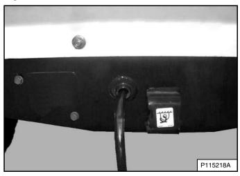
Pump the fluid out of the chaincase [Figure 258]. (Lift arms shown raised for visual clarity.)
