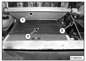
Pivot the air conditioning condenser (Item 1) up and rotate the support bar (Item 2) into position. Use low air pressure or water pressure to clean the top of the hydraulic fluid cooler and radiator assembly (Item 3) **[Figure 222]**.
