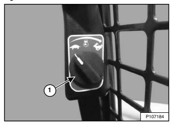
The engine speed control (Item 1) [Figure 54] is located alongside the door frame below the right panel.
