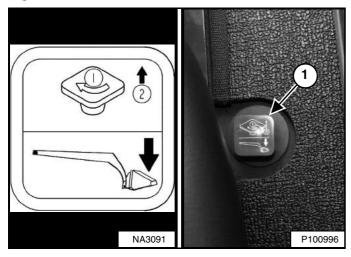
The lift arm bypass control (Item 1) **[Figure 57]**, located to the right of the operator's seat, is used to lower the lift arms if the lift arms cannot be lowered during normal operations.
