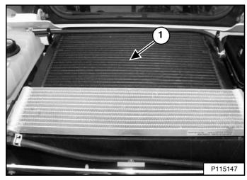
Use low air pressure or water pressure to clean the top of the hydraulic fluid cooler and radiator assembly (Item 1) **[Figure 224]**.
