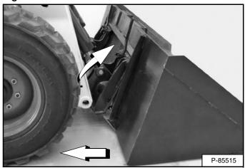
Tilt the Bob-Tach forward and drive the loader backward, away from the bucket or attachment [Figure 144].
