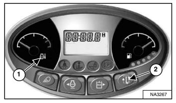
Frequently monitor the temperature and fuel gauges and BICS<sup>™</sup> lights (all BICS<sup>™</sup> lights must be OFF to operate loader) [Figure 133].
