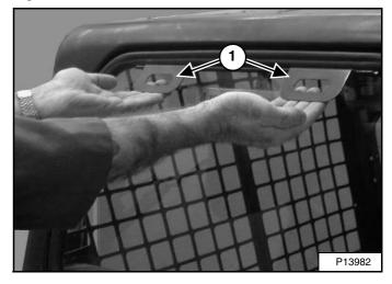
Pull both handles (Item 1) [Figure 65] up and out to remove the rear window.
