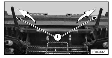
Push and <u>hold</u> BOB-TACH WEDGES "UP" switch (Right Switch Panel) [Figure 145] until levers (Item 1) [Figure 146] are fully raised (wedges fully raised). Figure 147
