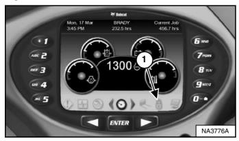
1. Press a scroll button repeatedly until the machine settings icon (Item 1) [Figure 36] is highlighted.
