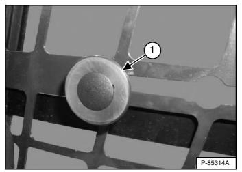
Pull the knob (Item 1) **[Figure 26]** and slide backward to open window. Release knob at cutout to lock in desired position. Pull the knob and slide forward to close window.
