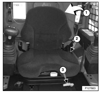
The switch (Item 1) **[Figure 122]** to turn the heated seat ON or OFF is located behind the seat back on the left side.
