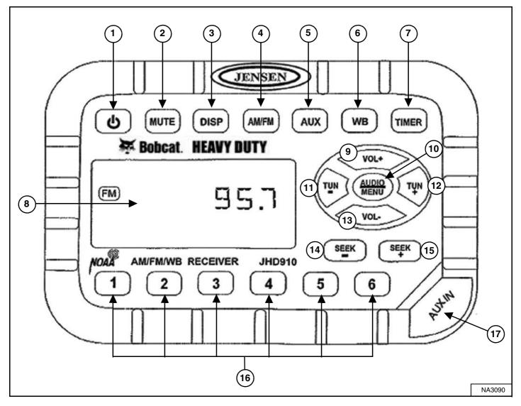
The table on the next page shows the DESCRIPTION and FUNCTION / OPERATION for each of the controls of the radio [Figure 18].
