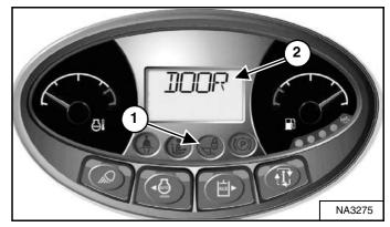
The LIFT AND TILT VALVE light (Item 1) **[Figure 179]** is OFF when the door is <u>closed</u>, the key switch is turned to RUN, the seat bar is lowered, and the PRESS TO OPERATE LOADER button is pressed.
