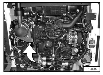
The air conditioning compressor is located behind the engine on the left side of the loader [Figure 264].
