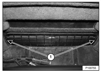
The recirculation filter is located behind the operator's seat inside the operator cab. The filter cover is held in position with three clips. Pull the cover at each end (Item 1) [Figure 191] to remove.
