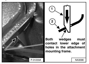
The wedges (Item 1) **[Figure 282]** must extend through the holes in the attachment mounting frame.
