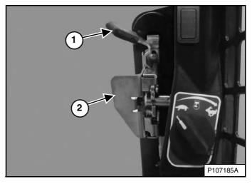
Pull the front door closed using the handle (Item 2) [Figure 28].
