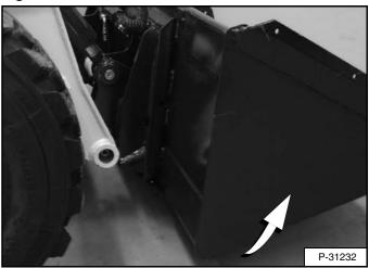
Tilt the Bob-Tach backward until the cutting edge of the bucket (or other attachment) is slightly off the ground **[Figure 148]**. This procedure will cause the bucket mounting frame to fit up against the front of the Bob-Tach.
