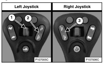
Additional switches (Items 1, 2, and 3) [Figure 115] or [Figure 116] are used to control some attachment functions through the attachment control device.
