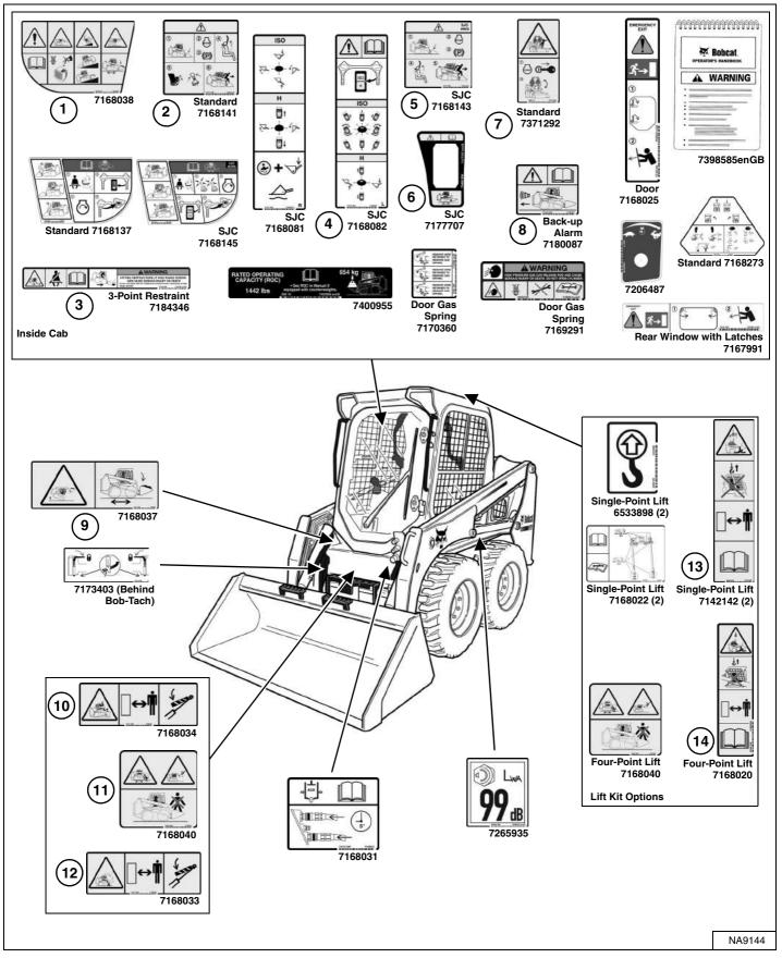
Follow the instructions on all the Machine Signs (Decals) that are on the loader. Replace any damaged machine signs and be sure they are in the correct locations. Machine signs are available from your Bobcat loader dealer.
