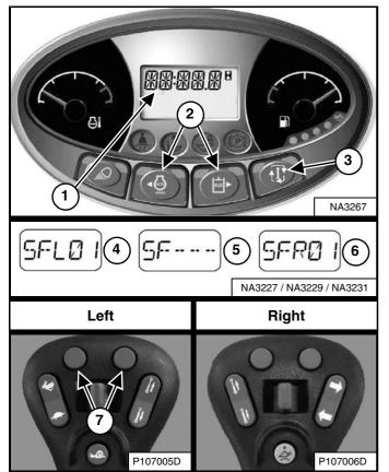
Press the Information button (Item 3) to cycle the data display until the steering drift compensation menu is displayed. The current steering drift compensation setting will appear in the data display (Item 1) [Figure 88].
