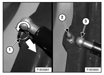
Rotate and pull the clip (Item 1) out of the gas spring socket. Pull the gas spring socket (Item 3) straight off the ball stud fitting (Item 2) **[Figure 68]**.
