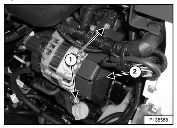
Remove the alternator belt shield mounting bolts (Item 1) [Figure 259].
