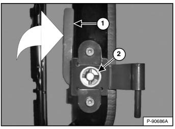
Install cast washers (Item 2) on door hinges taking care to match rectangular surfaces. Hold cast washer firmly against door and rotate latch (Item 1) **[Figure 70]** up to lock cast washer into position. (Bottom hinge shown.) (Plastic cap shown removed for visual clarity.)
