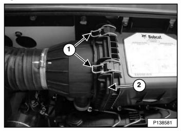
Install the cover (Item 2) and secure four latches (Item 1) **[Figure 203]**. (One latch is not visible in the photo.)
