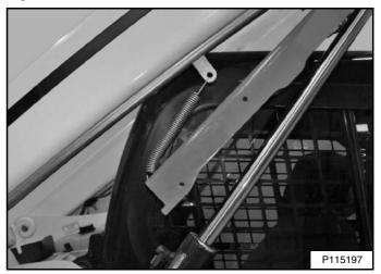
Raise the lift arms a small amount. The spring will lift the lift arm support device off the lift cylinder rod **[Figure 172]**. Fully lower the lift arms.
