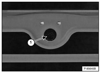
The back-up alarm (Item 1) [Figure 71] is located on the inside of the rear door.
