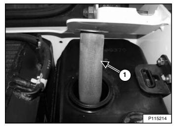
Remove and clean the hydraulic fill screen (Item 1) [Figure 248]. Use low air pressure to dry the screen.
