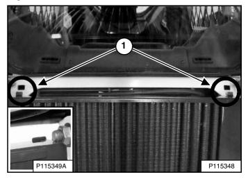
The front edge of the rear grille has two tabs that fit into slots in the loader frame (Item 1) **[Figure 189]**. Insert the tabs into the slots and lower the rear grille.
