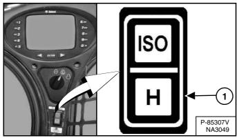
Select the 'H' control pattern by pressing the bottom of the switch (Item 1) [Figure 77].
