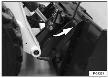
Drive the loader slowly forward until the top edge of the Bob-Tach is completely under the top flange of the bucket mounting frame **[Figure 147]** (or other attachment).
