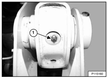
1. Lift Arm Pivot Pin (Both Sides) (2) [Figure 272].
