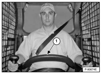
The seat bar restraint system has a pivoting seat bar with armrests (Item 1) [Figure 164].
