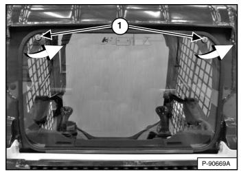
The rear window can be removed from outside the loader using a T40 TORX® Drive tool. Turn both screws (Item 1) [Figure 63] anticlockwise until the latches disengage from the window frame. Pull the top of the window away from the cab and lift up to remove.
