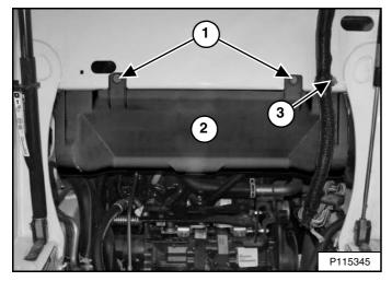
Remove the nut (Item 3) holding the operator cab electrical harness clamp and move the harness toward the front of the loader. Remove the bolts (Item 1) and remove the lower fan duct (Item 2) [Figure 262].
