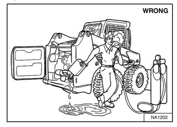
Use a clean, approved safety container to add fuel of the correct specification. Add fuel only in an area that has free movement of air and no open flames or sparks. *NO SMOKING* [Figure 205].
