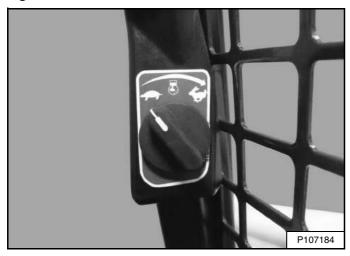
Set the engine speed control to the low idle position [Figure 128].
