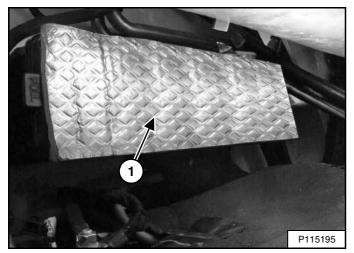
The electrical system is protected from overload by fuses located under the fuse panel cover (Item 1) [Figure 232]. Remove the fuse panel cover by pulling at each end.
