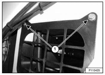
Remove the left side access cover bolts (Item 1) [Figure 246] and remove the access cover.
