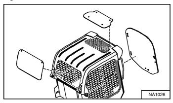
Available for special applications to restrict material from entering cab openings. Kit includes 12,7 mm (0.5 in) thick polycarbonate front door and polycarbonate rear window [Figure 4].
