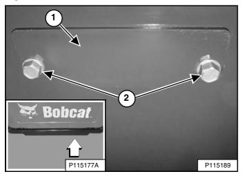
The oil drain hose is located behind a cover (Item 1) under the rear of the loader (Inset) **[Figure 215]**.
