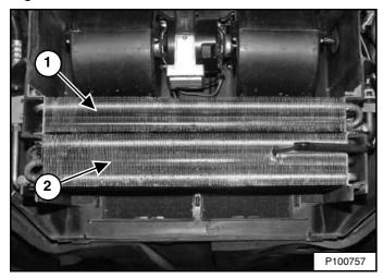
Use low pressure air or water to remove debris from the heater coil (Item 1) and evaporator (Item 2) [Figure 193].
