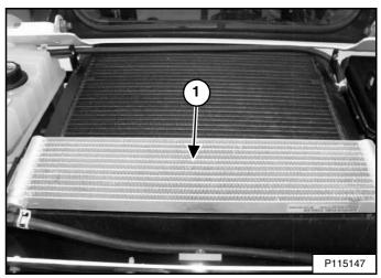
Use low air pressure or water pressure to clean the top of the fuel cooler (Item 1) [Figure 220].
