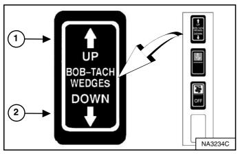
Push and hold the BOB-TACH WEDGES "UP" switch (Item 1) until wedges are fully raised. Push and hold the BOB-TACH WEDGES "DOWN" switch (Item 2) [Figure 284] until the wedges are fully down.
