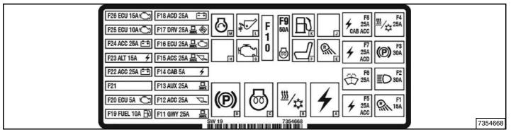
**SJC** - Fuse location and amperage ratings are shown in the table below and on the decal [Figure 236]. Relays are identified by the letter "R" in the AMP column.
