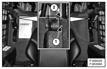
Use compressed air to clean any debris or dirt from the pivot parts. Do not lubricate. Inspect all mounting hardware. The correct hinge nut (both sides) (Item 1) torque is 34 - 38 N•m (25 - 28 ft-lb). The seat bar sensor nut (left side only) (Item 2) [Figure 165] torque is 6 - 8 N•m (50 - 70 in-lb).
