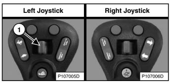
Move the Rear Auxiliary Hydraulic switch (Item 1) **[Figure 111]** or **[Figure 112]** to the left and right several times. Turn the key switch to STOP.
