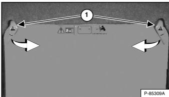
Turn both latches (Item 1) **[Figure 59]** in until they disengage from the window frame.
