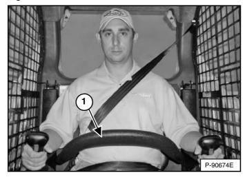
The Bobcat Interlock Control System (BICS<sup>TM</sup>) has a pivoting seat bar with armrests (Item 1) [Figure 32]. The operator controls the use of the seat bar.
