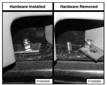
Remove the nuts and washers [Figure 181] (both sides) at the front corners of the operator cab.
