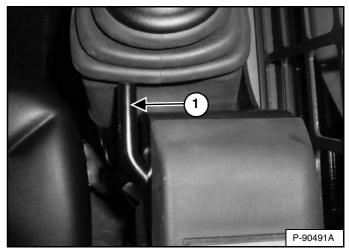
Pull the joystick adjustment lever (Item 1) [Figure 127] up to slide the loader joystick forward or backward to adjust for comfortable operation. (Right side shown.)
