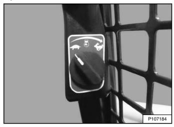
Set the engine speed control to the low idle position [Figure 134].
