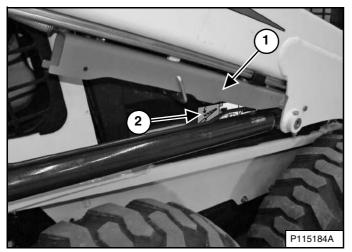
The lift arm support device (Item 1) **[Figure 167]** is used to support the lift arms while working on a machine with the lift arms up.
