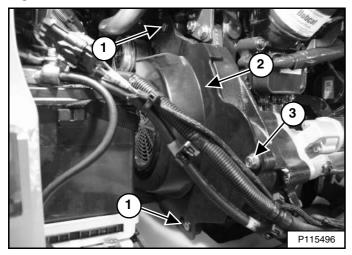
Remove the drive belt shield bolt (Item 3) [Figure 267].
