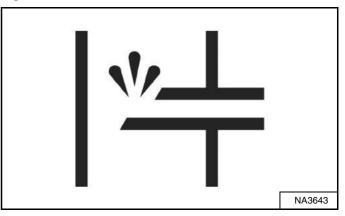
Wait for the fuel priming in process icon [Figure 208] on the right panel to turn off.
