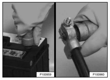
Always clean the battery terminals and cable ends when installing a new or used battery [Figure 241].
