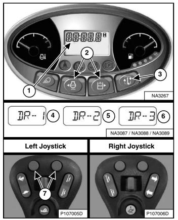
Press the Information button (Item 3) to cycle the data display until the drive response menu is displayed. The current drive response setting will appear in the data display (Item 1) [Figure 86].
