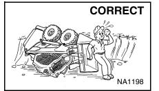
Never use loader without operator cab with ROPS and FOPS approval. Fasten your seat belt.
