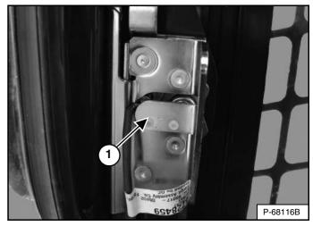
The cab door has a sensor (Item 1) **[Figure 178]** installed that deactivates the lift and tilt valves when the door is open.
