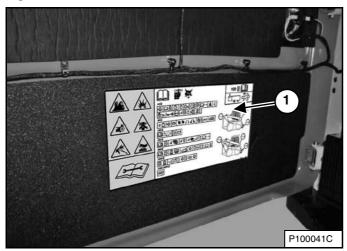
The Service Checklist And Schedule (Item 1) [Figure 117] is located inside the rear door of the loader.
