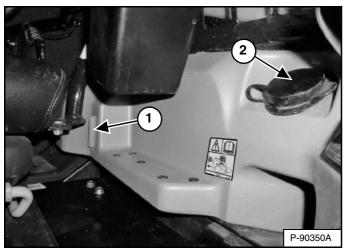
The washer fluid tank is located to the left of the operator seat. Check the fluid level in the sight gauge (Item 1). Remove the cap (Item 2) **[Figure 30]** to add washer fluid.
