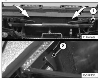
Push and <u>hold</u> BOB-TACH WEDGES "DOWN" switch (Right Switch Panel) [Figure 150] until levers are fully engaged in the locked position [Figure 151] (wedges fully extended through the attachment mounting frame holes).
