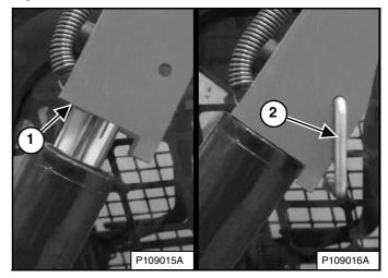
Raise the lift arms until the lift arm support device drops onto the lift cylinder rod (Item 1) [Figure 170].
