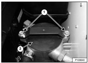
Loosen the bolts (Item 1) and rotate the filter cap (Item 2) **[Figure 249]** anticlockwise until the cap clears the bolts.
