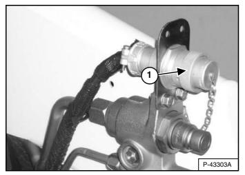
You will need the 14-Pin Attachment Control Device kit (Item 1) **[Figure 114]** to operate earlier model attachments. See your Bobcat loader dealer.
