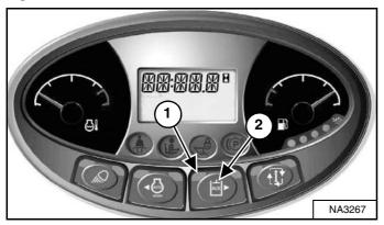
Press the Auxiliary Hydraulics button (Item 2) **[Figure 105]** once to activate the auxiliary hydraulics.
