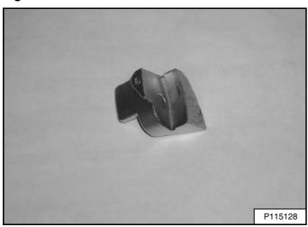
A belt tool **[Figure 261]** is required to install the new air conditioning belt. See your Bobcat dealer.
