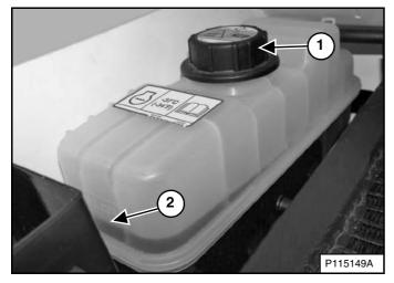
Remove the coolant fill cap (Item 1) [Figure 229] to drain the coolant faster.
