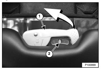
The lever (Item 1) is used to adjust the suspension response of the seat depending on the operator's weight. The optimum setting is achieved with the needle (Item 2) **[Figure 121]** centred in the gauge with the operator normally seated.
