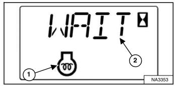
The machine will cycle the glow plugs automatically based on temperature. The engine preheat icon (Item 1) and the cycle time remaining or **[WAIT]** (Item 2) **[Figure 130]** are displayed in the data display.
