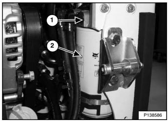
Remove the fuel filter element (Item 2) from the fuel filter head (Item 1) [Figure 211].
