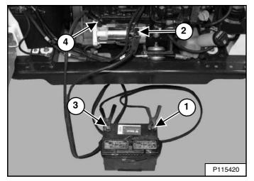
Connect the end of the first cable (Item 1) to the positive (+) terminal of the booster battery. Connect the other end of the same cable (Item 2) **[Figure 239]** to the positive (+) terminal on the engine starter.
