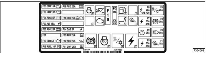
**Standard Controls -** Fuse location and amperage ratings are shown in the table below and on the decal **[Figure 235]**. Relays are identified by the letter "R" in the AMP column.
