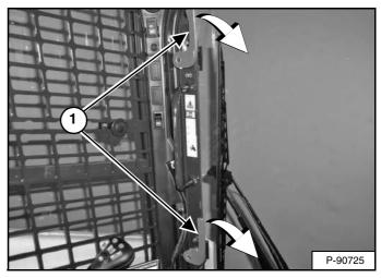
Turn both latches (Item 1) [Figure 66] down until they disengage from the door frame.
