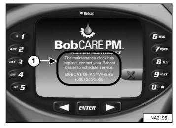
The Deluxe Instrumentation Panel will display a message (Item 1) **[Figure 291]** alerting the operator to service the machine.
