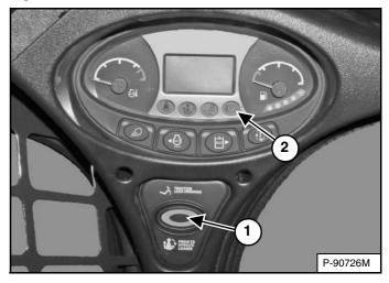
(Functions Only When The Seat Bar Is Raised And The Engine Is Running) There is a TRACTION LOCK OVERRIDE button (Item 1) [Figure 53] on the left instrument panel that will allow you to use the steering controls to move the loader forward and backward when using the backhoe attachment.
