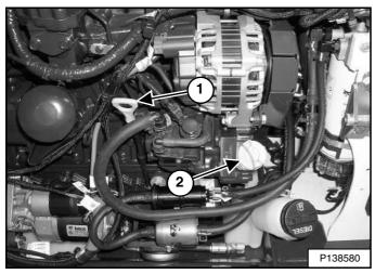
Park the loader on a level surface. Stop the engine. Open the rear door and remove the dipstick (Item 1) **[Figure 213]**.
