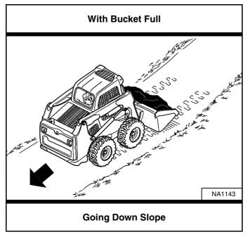
With a full bucket, go up or down the slope with the heavy end toward the top of the slope **[Figure 154]** and **[Figure 155]**.
