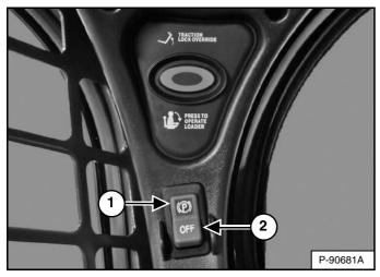
Press the top of the switch (Item 1) **[Figure 52]** to engage the parking brake. The red light in the switch will turn ON. The traction drive system is locked.
