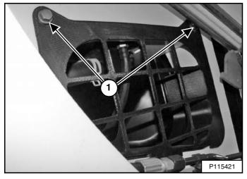
Remove the right side access cover bolts (Item 1) [Figure 245] and remove the access cover.
