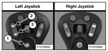
Adjust the speed percentage higher (Item 2) or lower (Item 3) **[Figure 84]** by pressing the Speed Control switch until the desired default setting is displayed.
