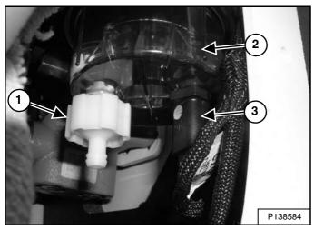
Attach a 9 mm (3/8 in) hose to the drain (Item 1) **[Figure 209]** at the bottom of the main fuel filter. Route the other end of the hose to a container.
