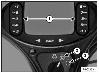
Turn the key switch to RUN (Item 2). The indicator lights on the left instrument panel will come ON briefly and the instrument panel / monitoring system will perform a self test. Use the numeric keypad (Item 1) [Figure 129] to enter the password.
