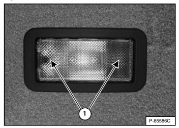
Push either side of the lens (Item 1) [Figure 31] to turn the light ON. Return the lens to the middle position to turn the light OFF.
