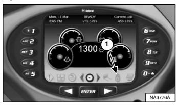
1. Press a scroll button repeatedly until the machine settings icon (Item 1) [Figure 40] is highlighted.
