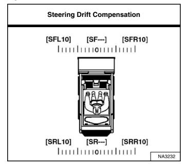
Steering drift compensation contains a total of 21 settings. Steering drift compensation can be set to any point from NEUTRAL to [SFL10] or [SRL10] left, and from NEUTRAL to [SFR10] or [SRR10] right. [SF---] or [SR---] is displayed when set for NEUTRAL [Figure 87].
