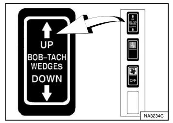
Push and <u>hold</u> BOB-TACH WEDGES "UP" switch (Right Switch Panel) **[Figure 152]** until levers are fully raised (wedges fully raised).
