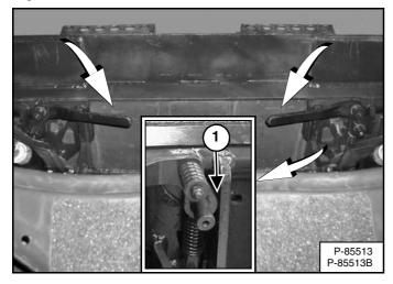
Push down on the Bob-Tach levers until they are fully engaged in the locked position [Figure 141] (wedges fully extended through the attachment mounting frame holes).
