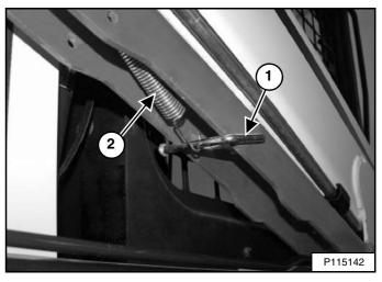
Raise the lift arm support device into the storage position and insert the retaining pin (Item 1) through the lift arm support device and the bracket. Hook the spring (Item 2) [Figure 173] to the retaining pin.
