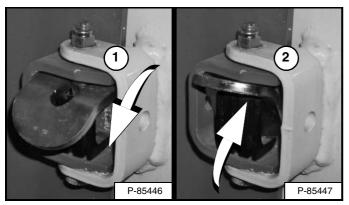
Move the door stop into the engaged position (Item 1) to hold the door open. Move the door stop up (Item 2) **[Figure 186]** to allow the door to close.
