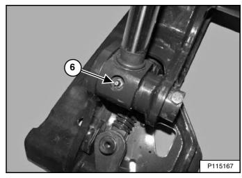
6. Rod End Tilt Cylinder (Both Sides) (2) [Figure 277].
