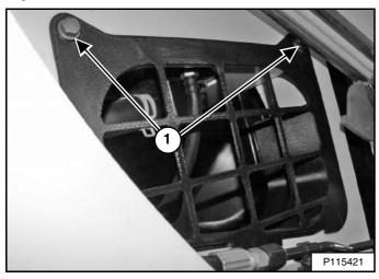
Remove the right side access cover bolts (Item 1) [Figure 251] and remove the access cover.
