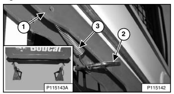
Put jackstands under the rear corners of the loader frame (Inset) [Figure 168].
