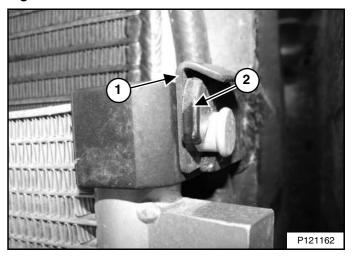
Ensure the air conditioning condenser is installed into the two slotted brackets (Item 2) [Figure 223]. (Right side shown.)
