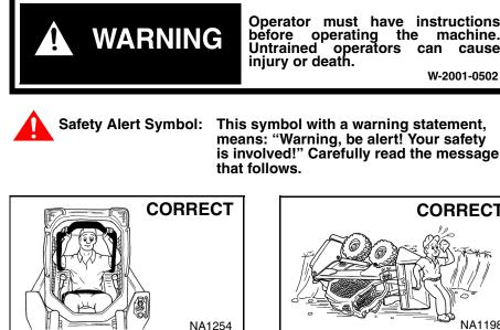
Always use the seat bar and fasten seat belt snugly. Always keep feet on the foot pedals or footrests when operating loader.
