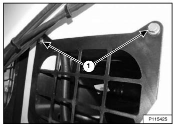
Remove the left side access cover bolts (Item 1) [Figure 263] and remove the access cover.
