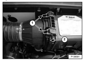
Open four latches (Item 1) and move the cover (Item 2) **[Figure 200]** out of the way. (Two latches are not visible in the photo.)
