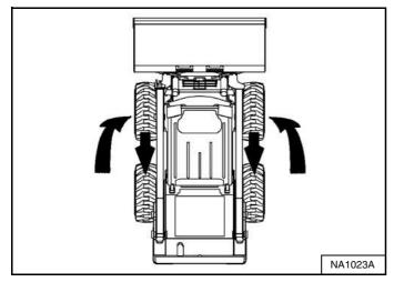
Rear tyres usually wear faster than front tyres. To keep tyre wear even, move the front tyres to the rear and rear tyres to the front **[Figure 256]**.
