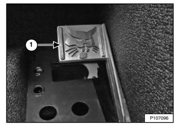
SJC equipped machines have a foot operated engine speed control pedal (Item 1) **[Figure 55]** in addition to the engine speed control knob. The pedal is located on the right side floor above the footrest.
