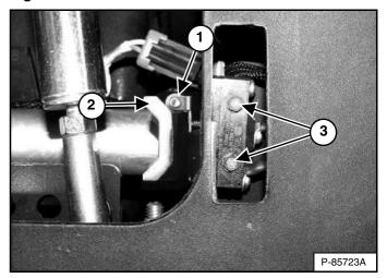
Loosen the screws (Item 3) **[Figure 177]** securing the back-up alarm switch. (Left side shown)
