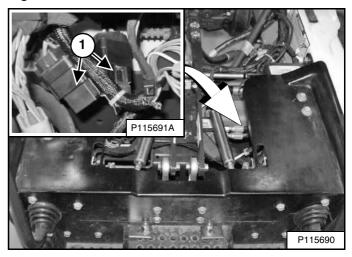
Two relays (Item 1) **[Figure 234]** for the loader lights are located under the operator cab on the left side of the loader. Stop the engine and raise the operator cab to access the relays. (See Raising on Page 134.)
