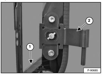
Orient the latches as shown (Item 1) and install the door hinges (Item 2) [Figure 69] on the door. (Bottom hinge shown.)
