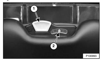
The lever (Item 1) is used to adjust the suspension response of the seat depending on the operator's weight. The optimum setting is achieved with the needle (Item 2) **[Figure 123]** centred in the gauge with the operator normally seated.
