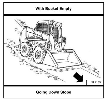
With an empty bucket, go up or down the slope with the heavy end toward the top of the slope [Figure 156] and [Figure 157].
