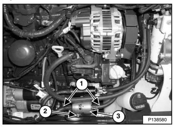
Pinch off the two hoses (Item 1) to prevent spilled fuel while the hoses are disconnected from the pre-filter (Item 3) **[Figure 207]**.
