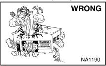
Do not use loader in atmosphere with explosive dust, explosive gas, or where exhaust can contact flammable material.
