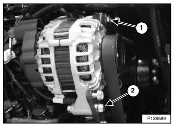
Loosen the top alternator mounting bolt (Item 1). Remove the bottom alternator mounting bolt (Item 2) **[Figure 260]**.
