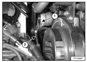
Insert a breaker bar (Item 2) into the square hole provided in the idler assembly (Item 1) [Figure 268] as shown and push the breaker bar down to release tension on the drive belt.
