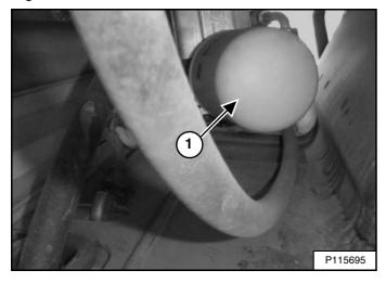
Put a suitable container below the filter, remove the filter (Item 1) **[Figure 252]**, and clean the filter base.
