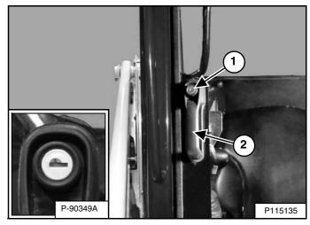
Push the knob (Item 1) and pull the handle (Item 2) to open the front door. A lock is provided in the knob (Inset) [Figure 27] to lock the front door when the loader is not in use.
