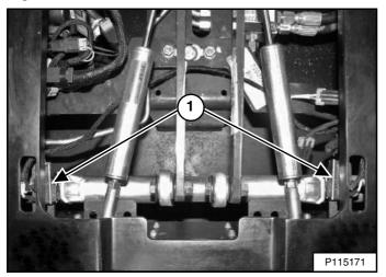
The back-up alarm switches (Item 1) **[Figure 176]** are located alongside the steering bellcranks. Both switches must be adjusted properly for the back-up alarm to operate correctly.
