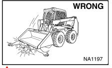
Never leave loader with engine running or with lift arms up. To park, engage parking brake and put attachment flat on the ground. CORRECT P-90216
