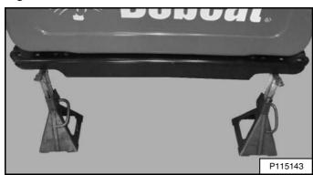
Install jackstands under the rear of the loader frame [Figure 180].
