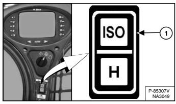
Select the 'ISO' control pattern by pressing the top of the switch (Item 1) [Figure 74].
