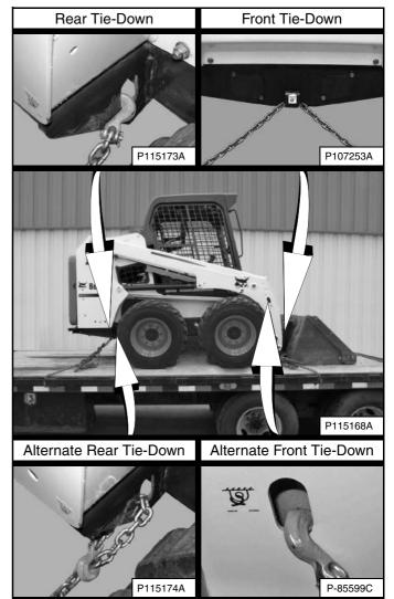
Use the following procedure to fasten the Bobcat loader to the transport vehicle to prevent the loader from moving during sudden stops, or when going up or down slopes **[Figure 162]**.
