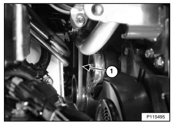
Cut the old belt (Item 1) **[Figure 265]** and remove the belt from the pulleys. Inspect the pulleys for wear.
