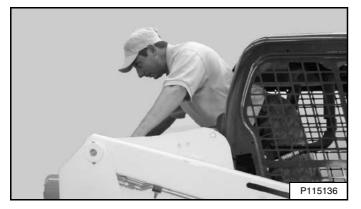
Exit through the rear of the operator cab [Figure 60].
