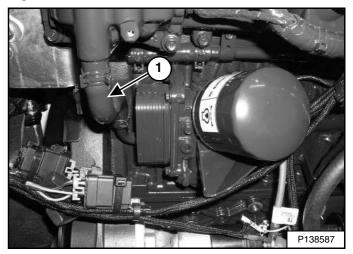
Pinch off the coolant hose attached to the engine oil cooler using a locking hose pinching plier or similar tool (Item 1) [Figure 228].
