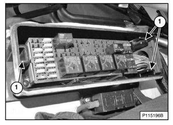
Line up the clips on the back of the fuse panel cover with the slots (Item 1) **[Figure 233]** in the fuse panel and push the cover into position when finished.
