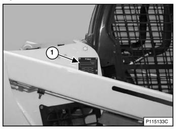
The loader serial number plate (Item 1) [Figure 1] is located on the outside of the loader frame.
