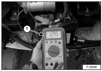
The simplest and most common check to determine battery state of charge is to use a digital multimeter or voltmeter (Item 1) [Figure 238].
