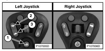
Press the button (Item 1) [Figure 82] on the left joystick once to engage Speed Management.
