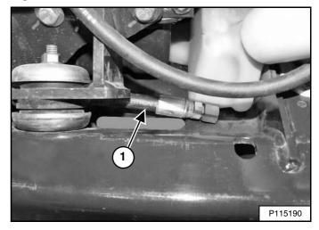
The oil drain hose (Item 1) **[Figure 216]** storage location is near the fuel tank fill. Route the oil drain hose through the opening.
