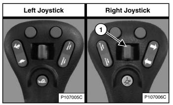
Move the Front Auxiliary Hydraulic switch (Item 1) [Figure 101] or [Figure 102] to the right or left to change direction of the auxiliary hydraulic fluid flow to the front quick couplers. If you move the switch halfway, the auxiliary functions move at approximately one-half speed. (EXAMPLE: Open and close grapple teeth.)
