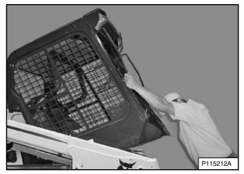
Lift on the grab handles and bottom of the operator cab **[Figure 182]** slowly until the operator cab is all the way up and the latching mechanism engages.
