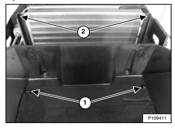
NOTE: The bosses (Item 1) fit inside the core supports (Item 2) [Figure 195] when the cover is installed. Deformity of the cover indicates they are out of position.
