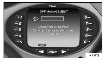
The machine will alert the operator when DPF service is required [Figure 254].
