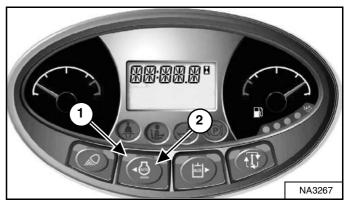
Press the button (Item 2) to engage auto idle. The light (Item 1) [Figure 56] is ON.
