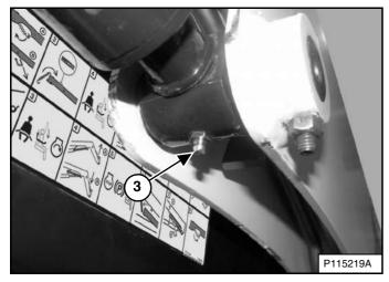
3. Rod End Lift Cylinder (Both Sides) (2) [Figure 274].
