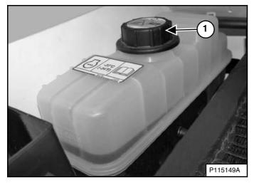
Remove the coolant fill cap (Item 1) [Figure 227].
