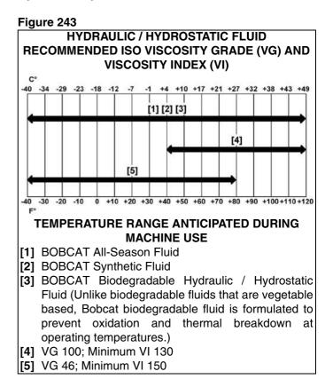
Bobcat hydraulic fluids are recommended for use in this machine. If Bobcat hydraulic fluid is not available, use a good quality hydraulic fluid meeting the viscosity grade and viscosity index shown in the chart [Figure 243].
