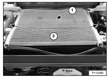
Use low air pressure or water pressure to clean the top of the air conditioning condenser (Item 1) [Figure 221].
