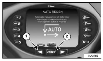
4. Press the **[ENTER]** button (Item 2) **[Figure 39]** to engage automatic mode.
