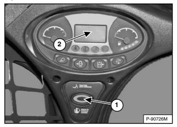
Press the PRESS TO OPERATE LOADER button (Item 1) **[Figure 132]** to activate the BICS<sup>™</sup> and to perform hydraulic and loader functions.
