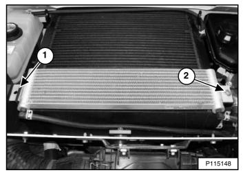
The area between the fuel cooler and the hydraulic fluid cooler and radiator assembly will require occasional cleaning. Remove the bolt (Item 2) and lift the fuel cooler up while sliding out of the bracket (Item 1) [Figure 225].
