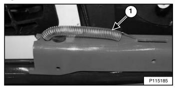
Lower the lift arm support device to the top of the lift cylinder. Hook the free end of the spring (Item 1) [Figure 169] to the lift arm support device to prevent interference with lift arm support device engagement.
