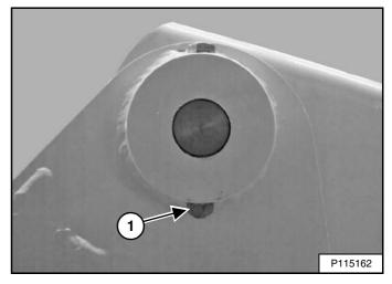
All lift arm and cylinder pivots have a large pin held in position with a retainer bolt and locknut (Item 1) **[Figure 280]**.
