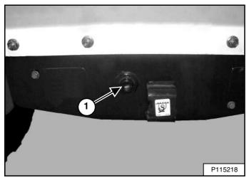
Remove the check plug (Item 1) [Figure 257] from the front of the chaincase housing. (Lift arms shown raised for visual clarity.)
