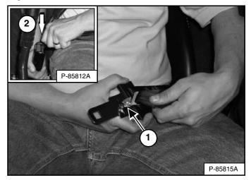
Connect the shoulder belt to the lap belt (Item 1). Pull the lap belt across to the right side of the seat and fasten (Item 2) [Figure 125].
