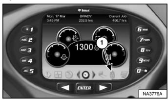
1. Press a scroll button repeatedly until the machine settings icon (Item 1) [Figure 44] is highlighted.
