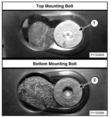
Position the drive belt shield over the drive belt shield mounting bolts. Slide the drive belt shield toward the front of the loader to fully seat the shield onto the top and bottom mounting bolts (Items 1 and 2) [Figure 269].
